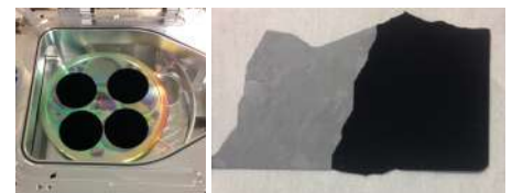
Fig. 3. Four wafers with B-Si (left). Comparison between two polycrystalline Si samples before and after B-Si step.
